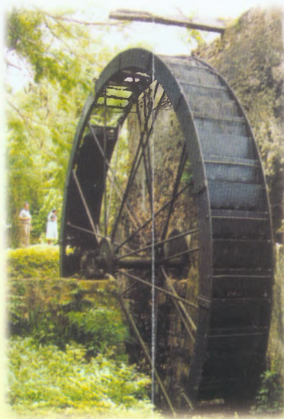
A water wheel used to power cane grinding operations at Seville.
